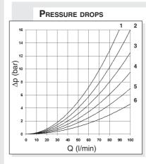
The diagram at the side show the pressure drop curves for spools during normal usage. The fluid used is a mineral oil with a viscosity of 46 mm<sup>2</sup>/s at 40°C; the tests have been carried out at a fluid
