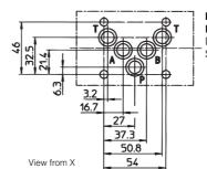
ISO 4401: 2005 Mounting surface: 4401-05-04-0-05 Diameter of ports A, B, P, T: Ø = 11,2 mm Seals: 5 OR 2050
